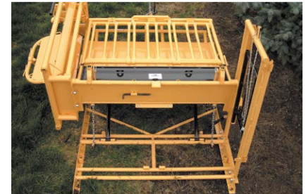
A vertical sliding tailgate stays upright when table is tipped to eliminate a separate gate to stop animals in alley.
