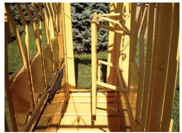
Body squeeze brings the animal to the operator's side.
