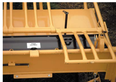
Adjustable leg pin for separating the animals legs for castrating.
