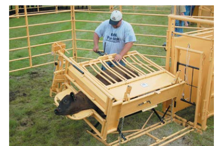
The table is equipped with a headboard to aid in head restraint and less stress while the animal is tipped on it's side.
