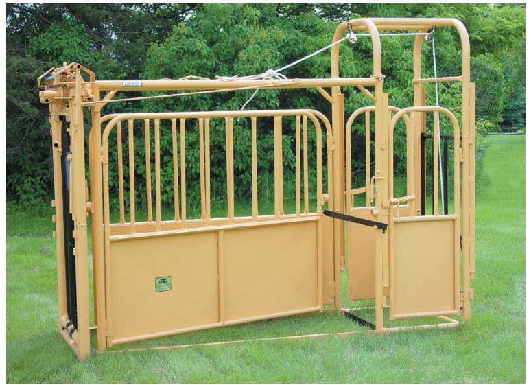
Ratchet bar squeeze adjustment holds animal in place.
